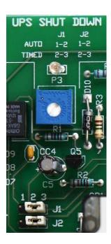
Regardless of the mode selected, this controller has an **LED** above **P3** that will be ON when the failsafe has been shut down after a power failure, and it will remain ON until normal power is restored.
